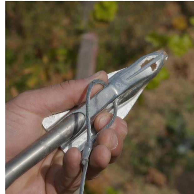
APEX anchor seated on Gripple Drive Tool.
